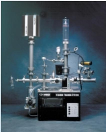
*A commercial high-vacuum training system with residual gas analysis capability.*
