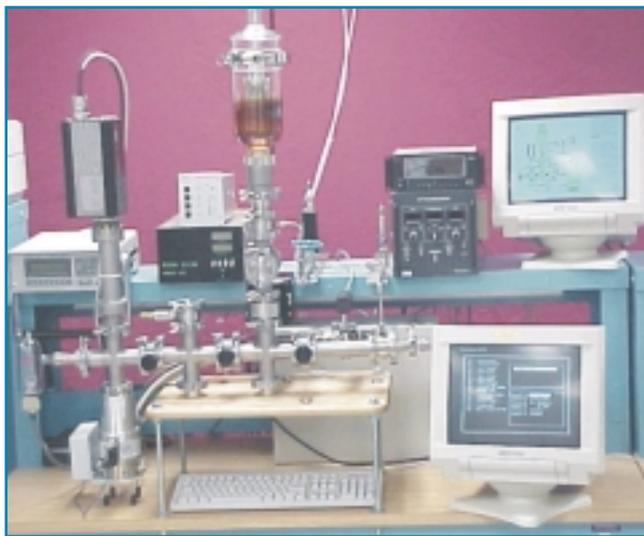
**Figure 5.** Automated system for sputter deposition of copper. Courtesy of Patrick McDonough, Weatherford Community College.
