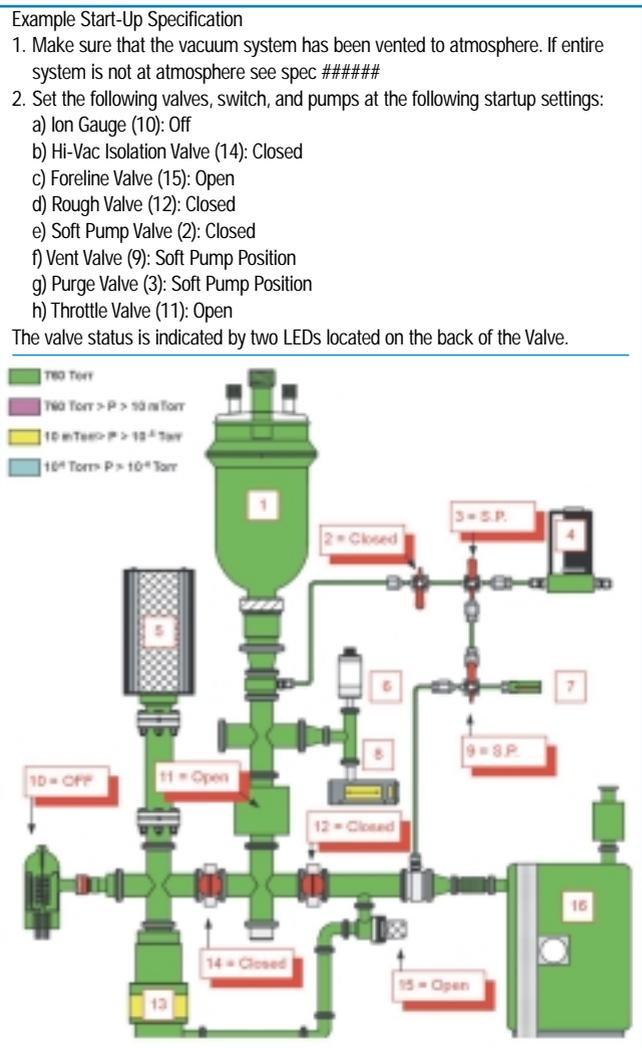
Figure 3. Portion of a Student Guide for start-up of a vacuum training system. Courtesy of Patrick McDonough, Weatherford Community College.
