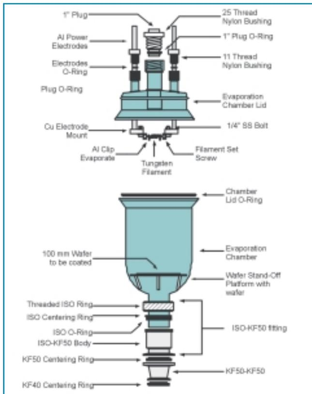
Figure 2. Components of evaporation module. Courtesy of Patrick McDonough, Weatherford Community College.
