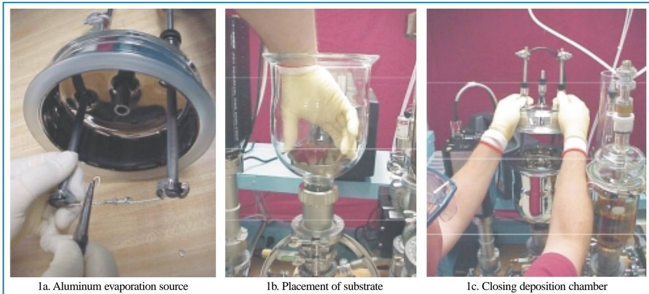
1a. Aluminum evaporation source      1b. Placement of substrate      1c. Closing deposition chamber
