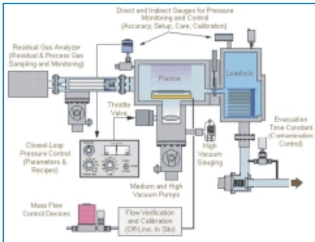
**Figure 4.** Simplified schematic diagram of a generic semiconductor process tool (plasma source not shown).
