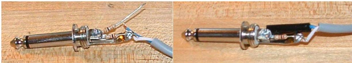
**Figure 2.** Voltage divider assembly.
