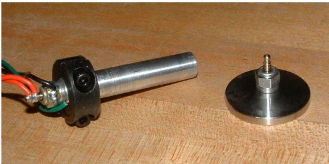
The above glow plug assemblies have the disadvantage of not rendering the filament visible. At low pressures, as the thermal conductivity of the residual gas reaches a minimum, the filament will glow. This is a useful visual aid.
