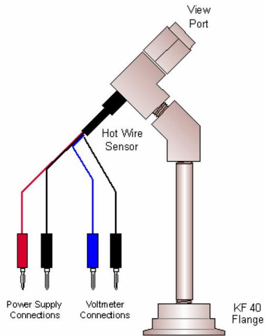
The fixture is made from ¼-inch brass pipe fittings. The right angle fitting is a pipe thread to compression (tubing) adapter. The tubing end is fitted with a small lens or other clear plastic or glass disk. It may be affixed and sealed with an o-ring or with epoxy. The position of the glow plug permits the filament to be seen through the window. Other permutations are, of course, possible.
