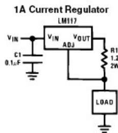
The prototype is shown in the picture below. Two leads (plug center pin and shank leak) are connected to the power supply via banana plugs/jacks. The other two leads (shown not connected) are either connected to a DVM or (better) to a Vernier voltage probe. I used resistors from a local supplier. Since they didn't have a 1.2 ohm resistor I used a 1 ohm in series with two 0.5 ohm in parallel. The resulting current was 1.001 ampere. Power is supplied by a 12 volt wall wart.
