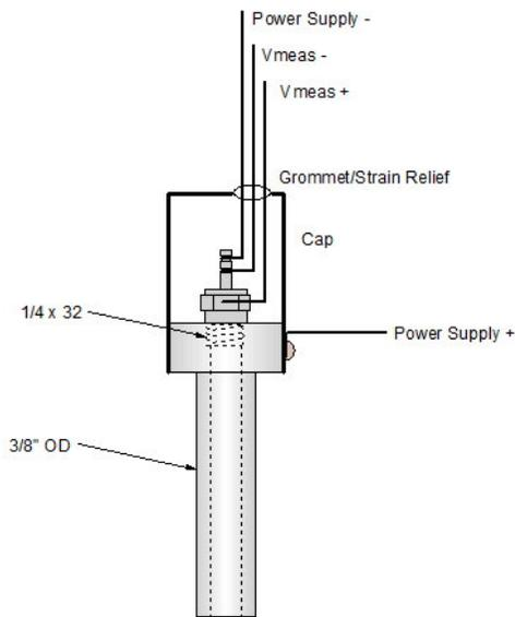
The starting material is rod stock, about 3 inches long. Using a small lathe, drill through the axis and tap one end deep enough for the glow plug's threads.
