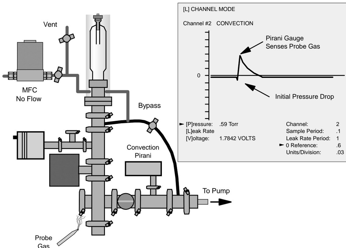
**Figure 43: Leak Detection Using the Pirani gauge**
