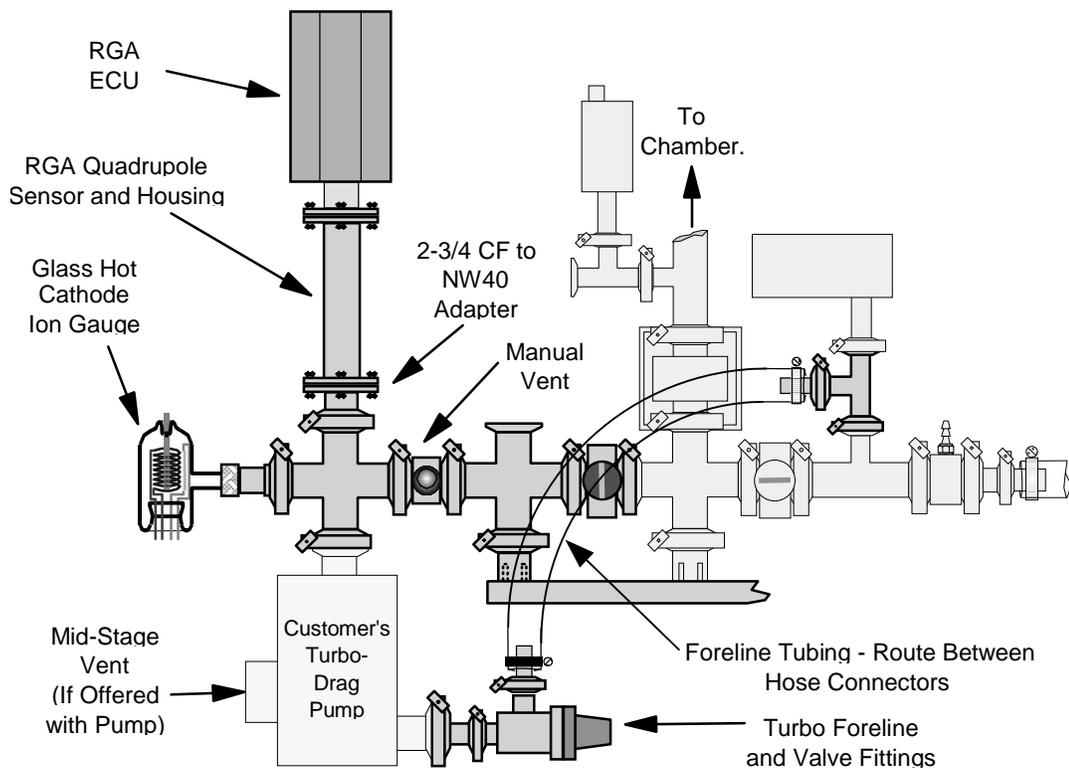
**Figure 49: Adding the High Vacuum Components**
