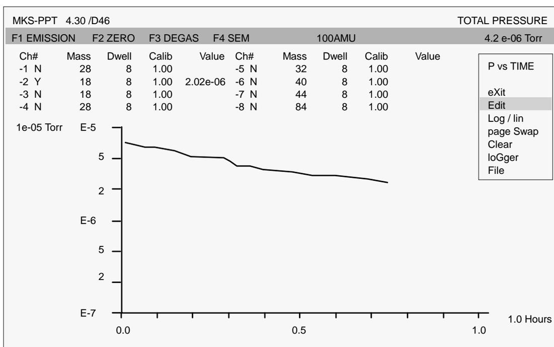
Figure 56: Pressure vs Time Mode Plot for Mass 18
