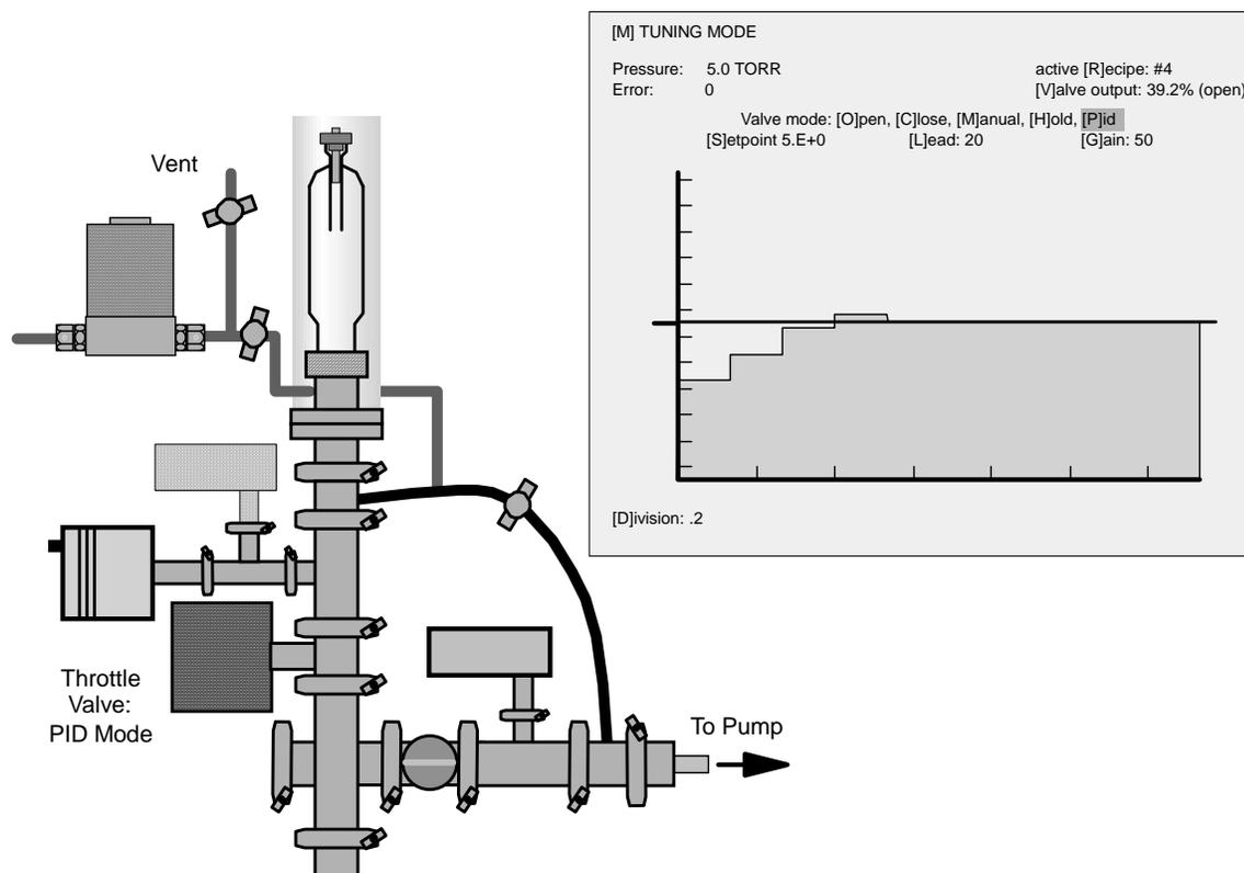
**Figure 32: Downstream Auto Pressure Control**
