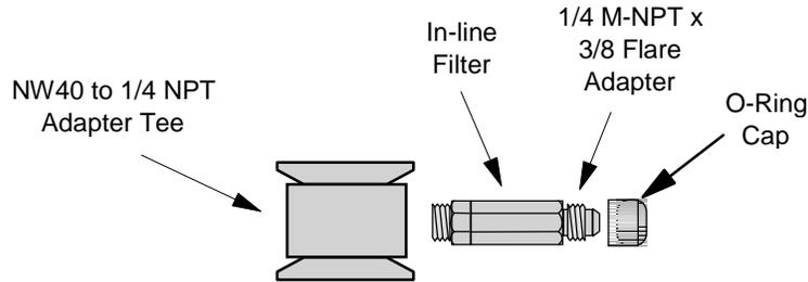
**Figure 48: Assembly of the Manual Vent**
