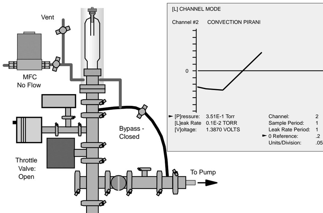
**Figure 25: Up Leak Check**
