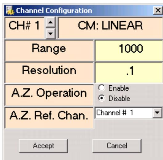
Figure 18: Channel #1 Configuration Settings
