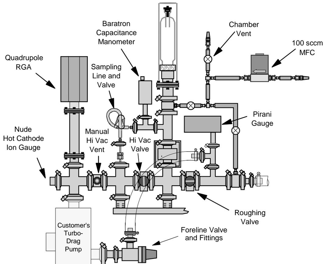
**Figure 51: Fully Assembled System (CE Compliant Version)**
