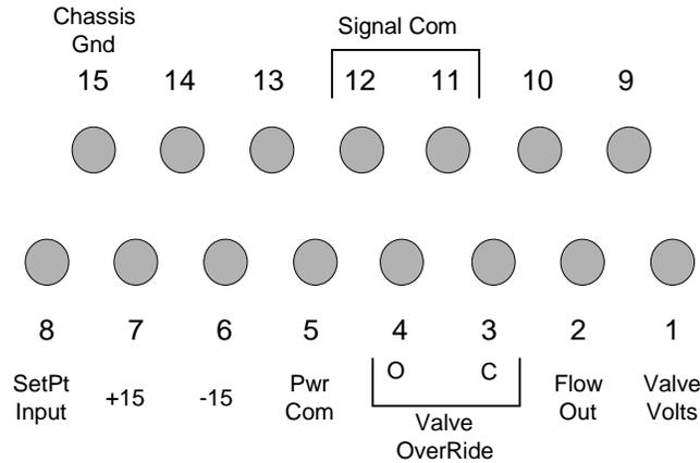
**Figure 41: Breakout Connector Pinout**
