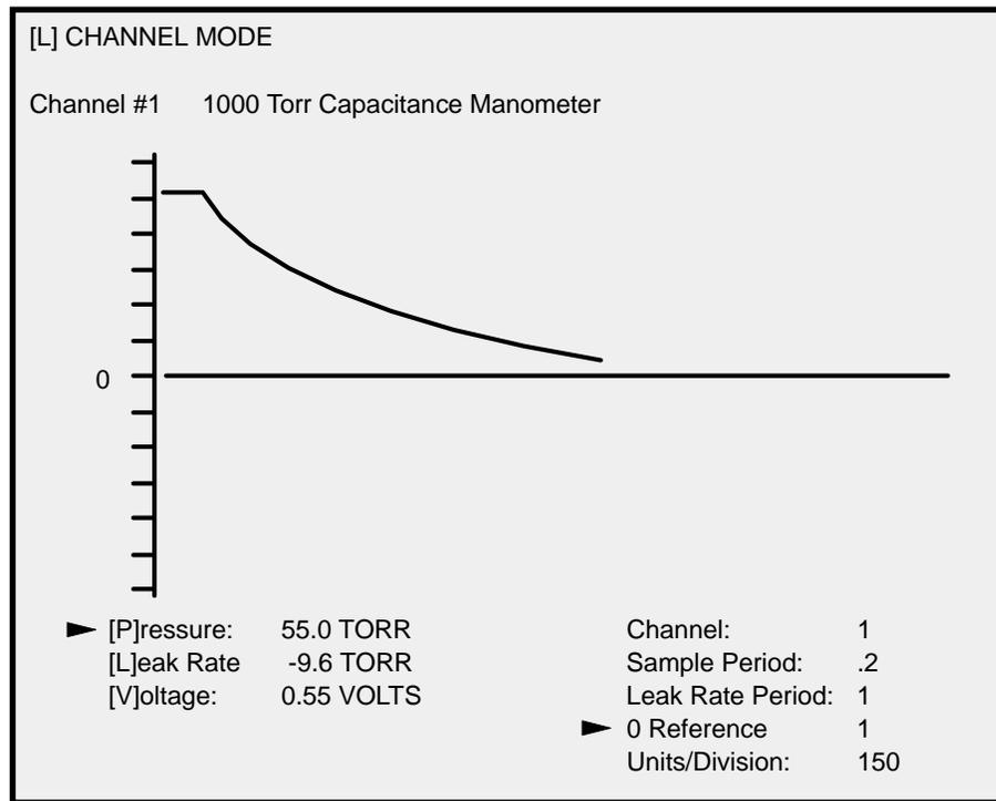
**Figure 11: RTI Channel Mode Screen**
