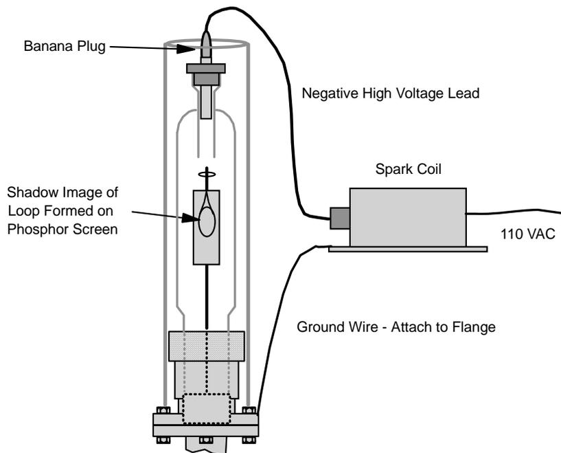
**Figure 46: Cold Cathode Electron Tube Assembly**
