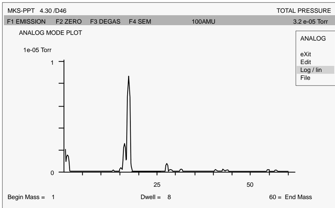
**Figure 52: Analog Mode Mass Scan with Linear Pressure Scale**
