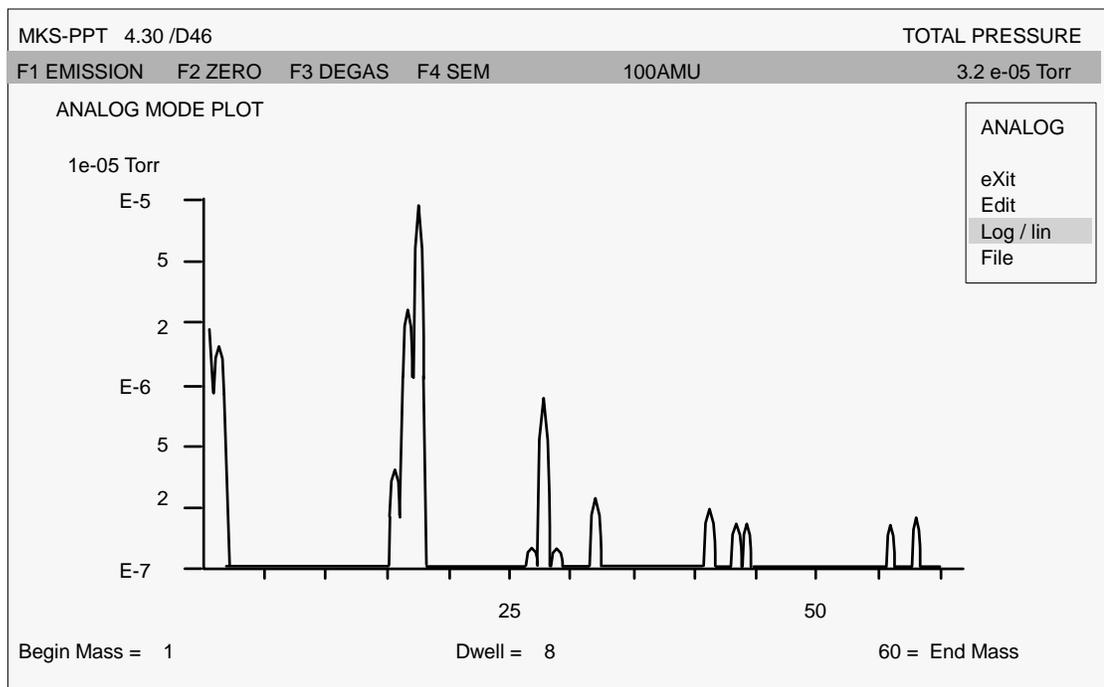
Figure 53: Analog Mode Mass Scan with Logarithmic Pressure Scale
