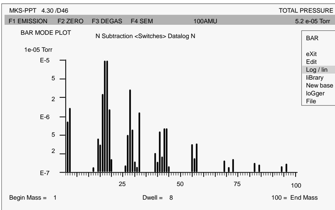
**Figure 54: Bar Mode Mass Scan with Logarithmic Pressure Scale**
