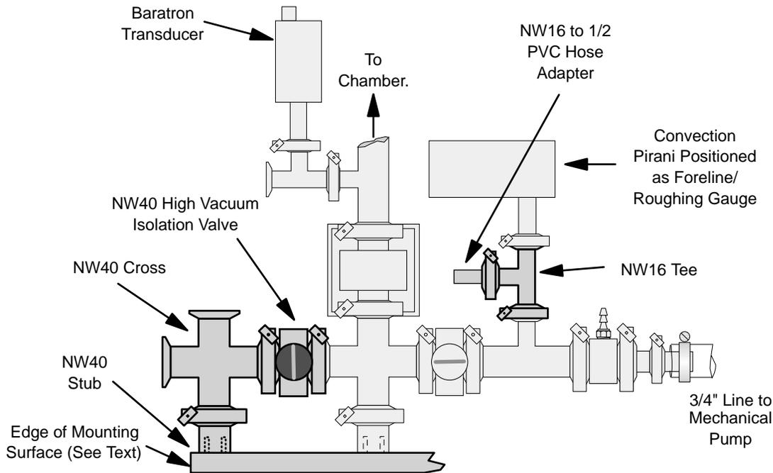
**Figure 47: Beginning the Assembly of the High Vacuum Manifold**
