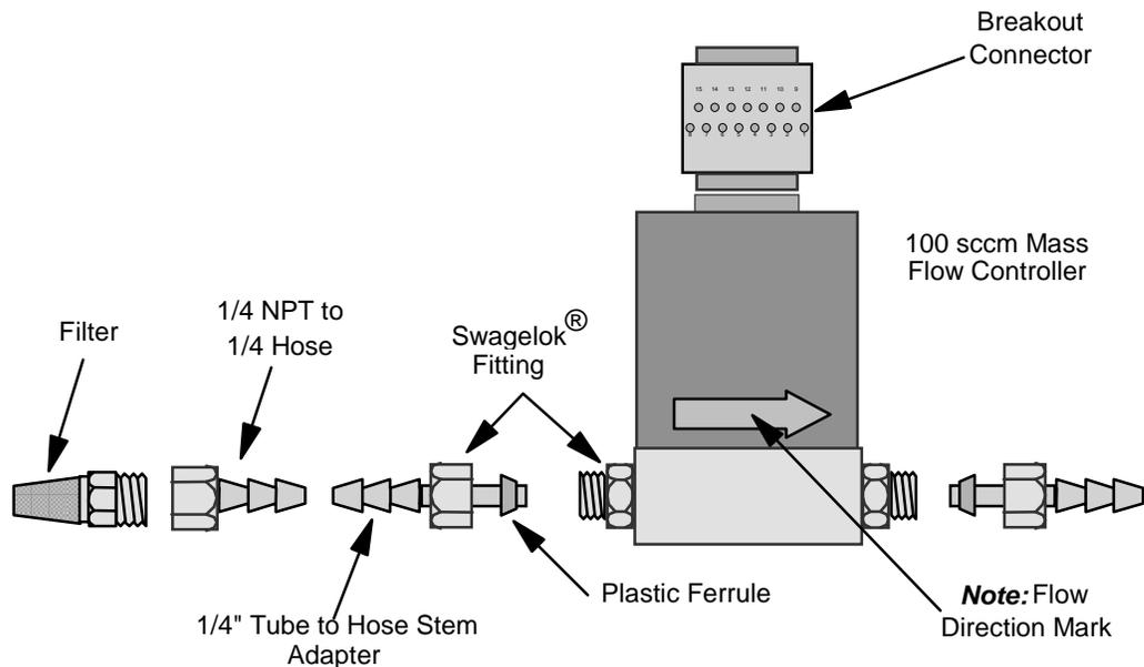
**Figure 5: Mass Flow Controller**
