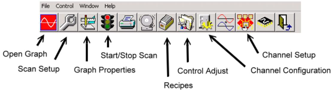
**Figure 14: Toolbar Showing Menu Items Used With the VTS-1B and 2A**
