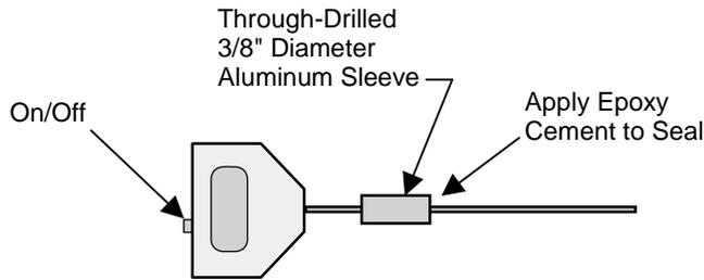
**Figure 7: Thermometer Assembly**
