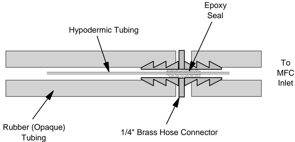
**Figure 42: Flow Constriction Device**
