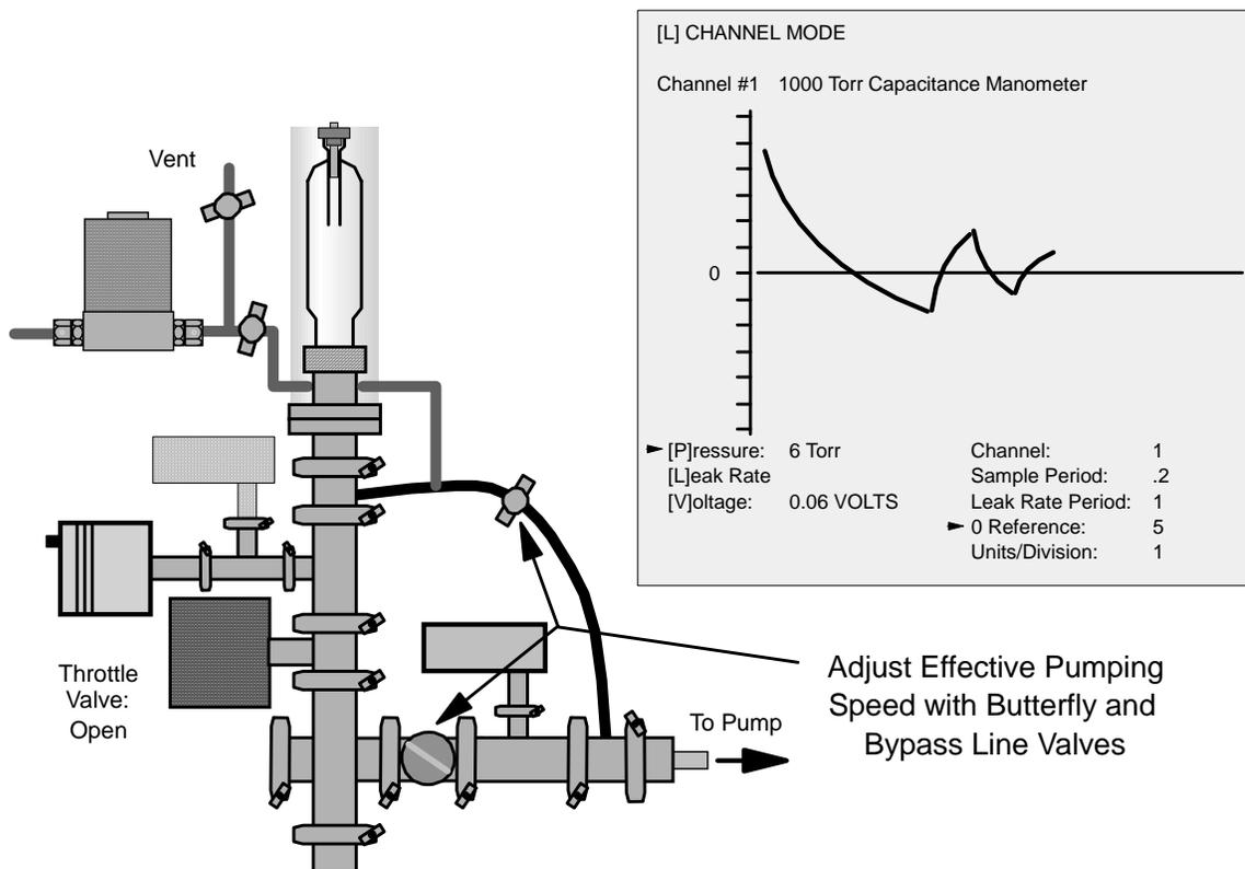
**Figure 31: Downstream Manual Pressure Control**
