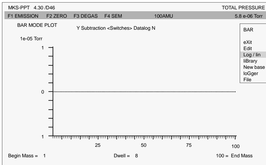
**Figure 58: Baseline Using the Subtraction Parameter**
