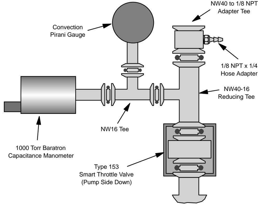
**Figure 2: Throttle Valve and Gauges**
