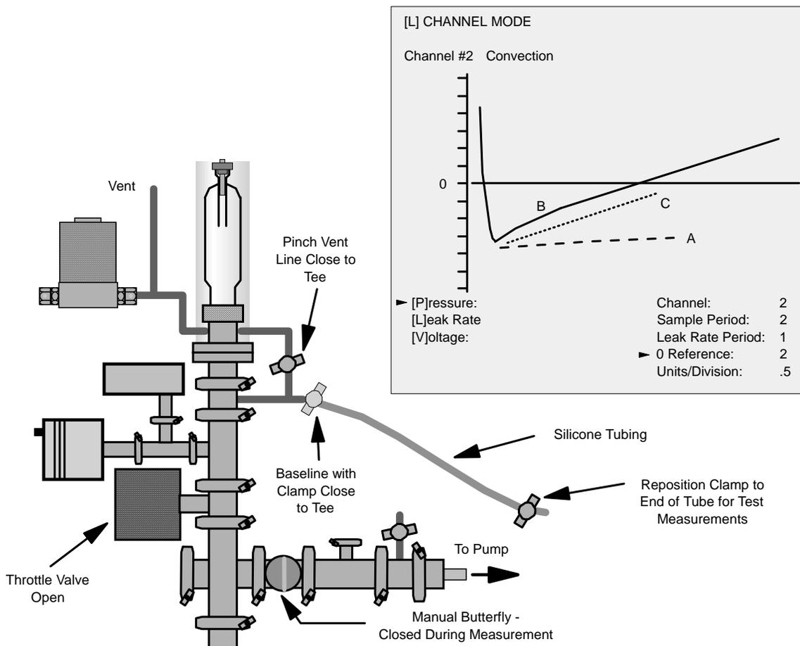
**Figure 44: Observing Outgassing and Permeation**
