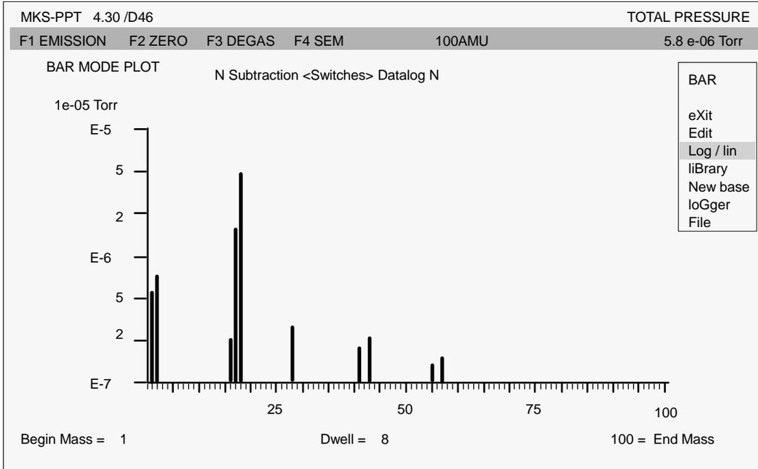
Figure 55: Bar Mode Mass Scan After Closing High Vacuum Valve
