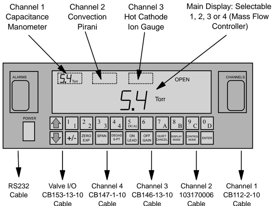
**Figure 8: The Front Panel of the 146 Instrument (VTS-1B Cabling is Shown)**
