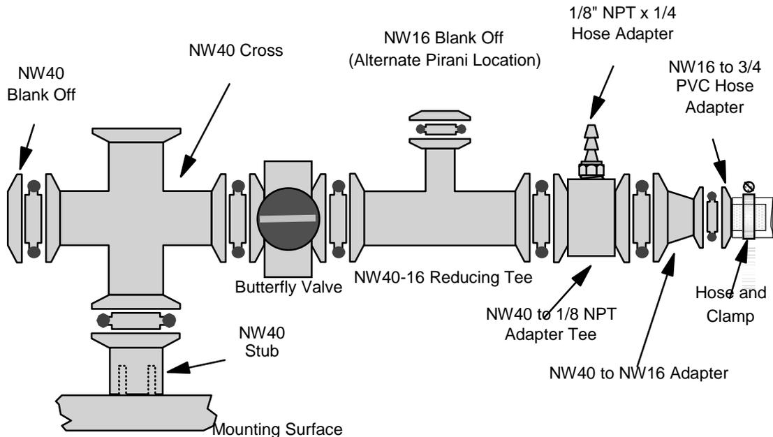
**Figure 1: Lower Manifold**
