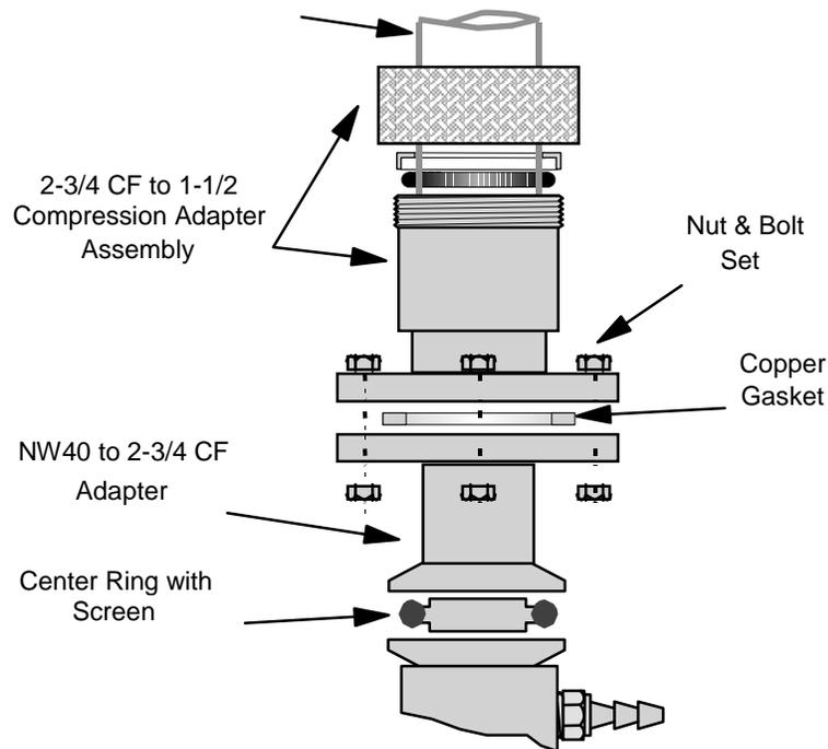
**Figure 3: CF & Compression Adapters and the Glass Chamber**
