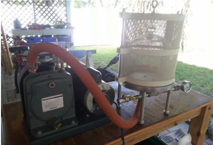
This vacuum system that was used only one time to de-bubble potting compound. Since then it has been in storage. It consists of the following items:
