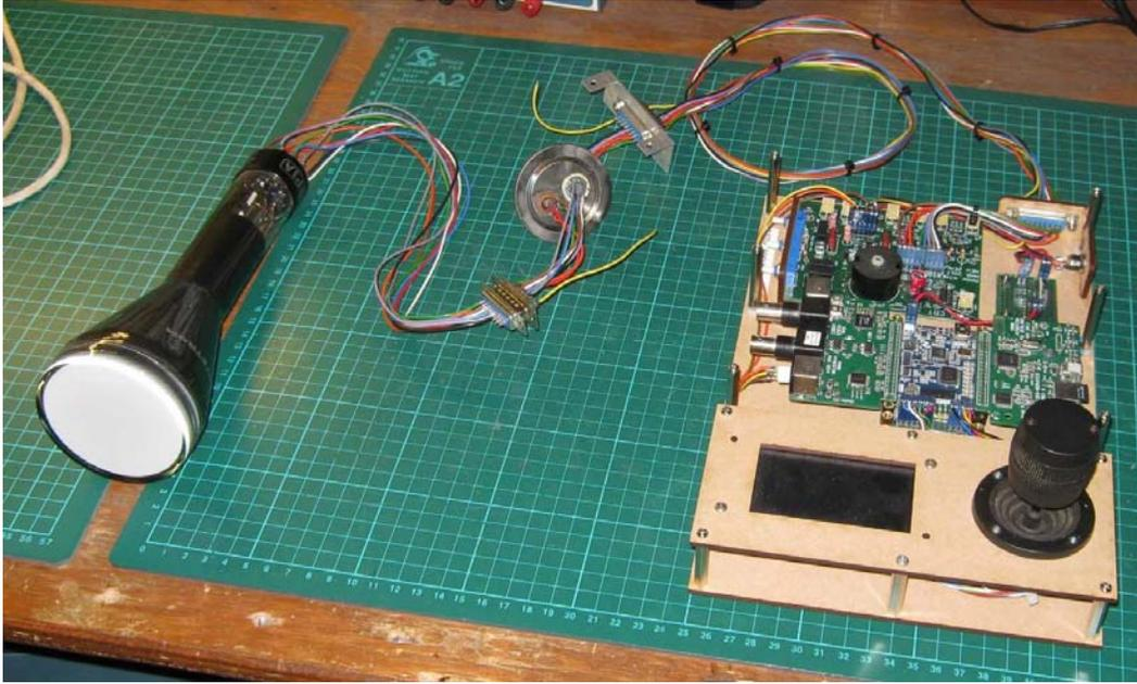
Custom test generator<sup>7</sup>, with 3RP1A CRT attached
