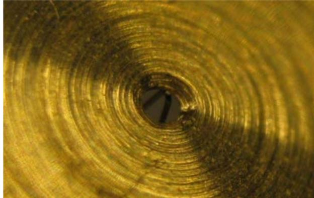
250 micron filament sitting slightly proud in a 700 micron hole.
