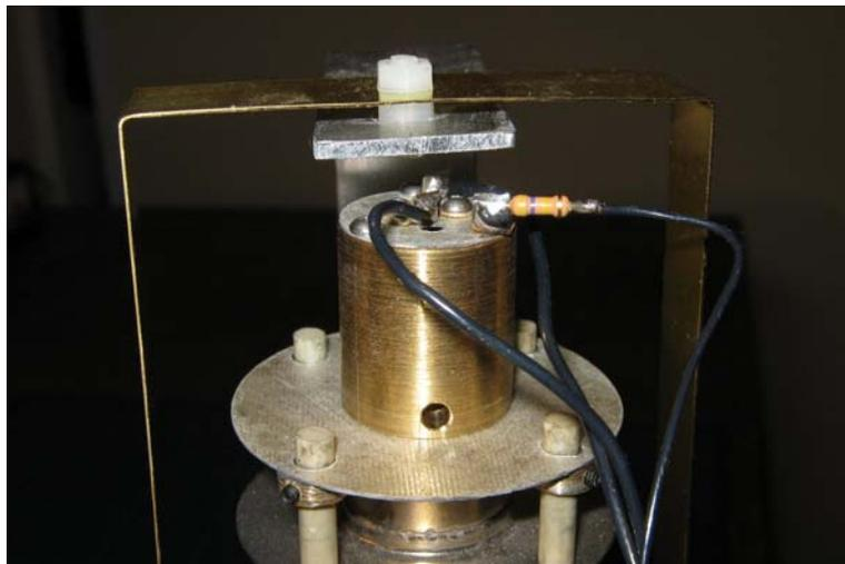
Laser cut front and rear mica disks providing interface to the focus assembly as well as electrical connection to the filament and G1 (with 470k resistor)
