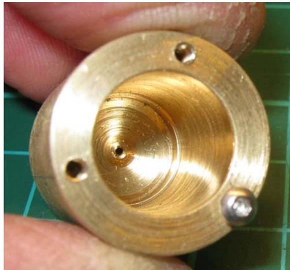
700 micron electron aperture at the base of the new Wehnelt cylinder
