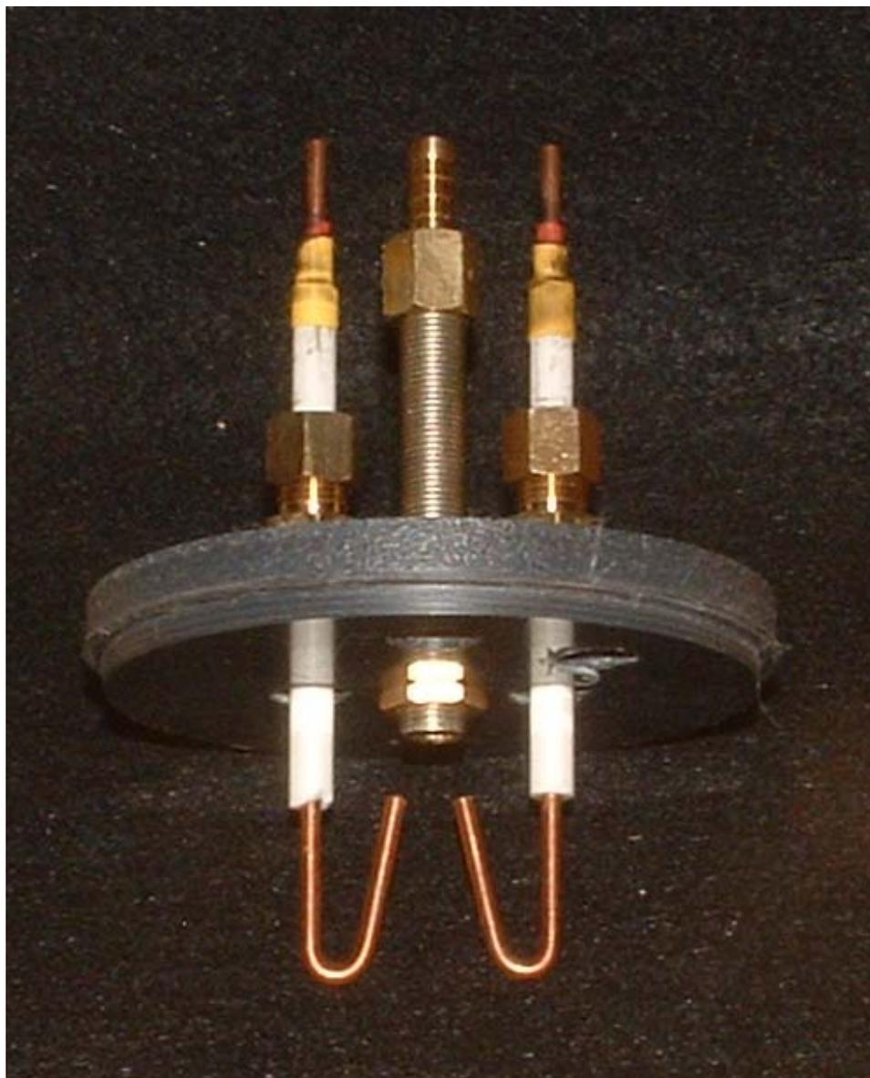
The port for the gas inlet is placed at the center. This was drilled and tapped for 1/8" pipe thread. In line and outboard of this are two holes for the electrode assemblies. These were drilled and tapped for 1/4" pipe thread with centers at 1-3/8" separation. I used 1/4 M-NPT x 1/4" brass compression fittings with Teflon inserts to hold the electrode assemblies.
