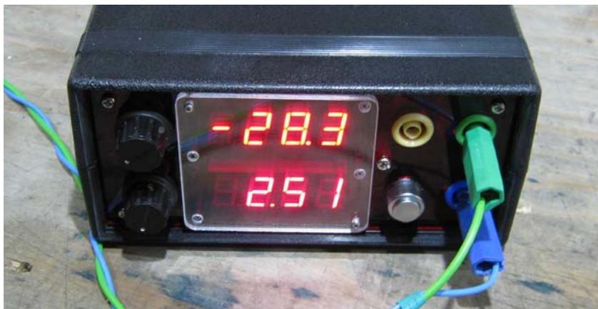
Homemade floating filament and grid supply
