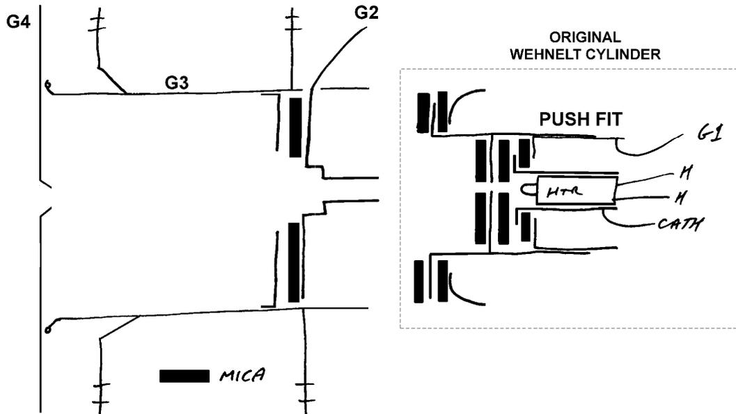
Original Wehnelt cylinder, and focus assembly
