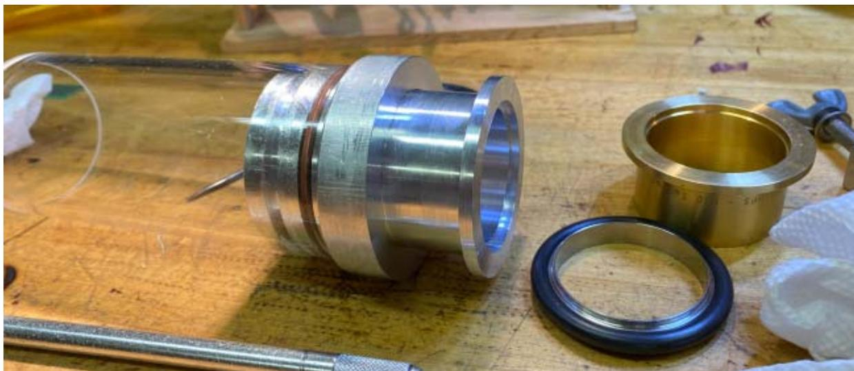
Additionally, having the glass bump up directly to the metal fitting can lead to cracks in the glass. A solution is to put a rubber “bumper” between the fitting flange and the tube.
