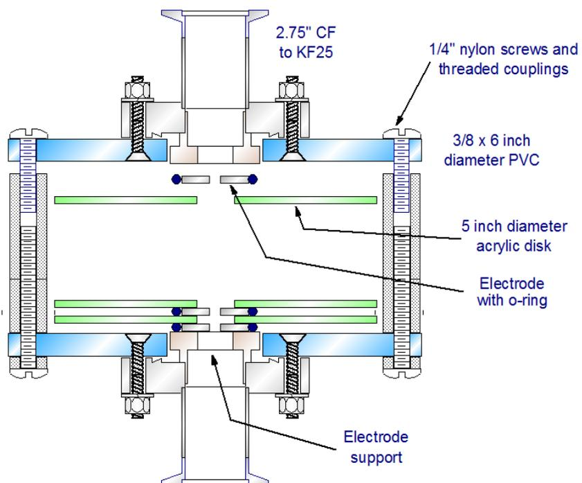
I cut out the PVC disks using a circle cutter in my drill press. The acrylic disks are available from US Plastic (<https://www.usplastic.com>) as part number 44187. I drilled a 1/2" hole at the center of each of the acrylic disks.
