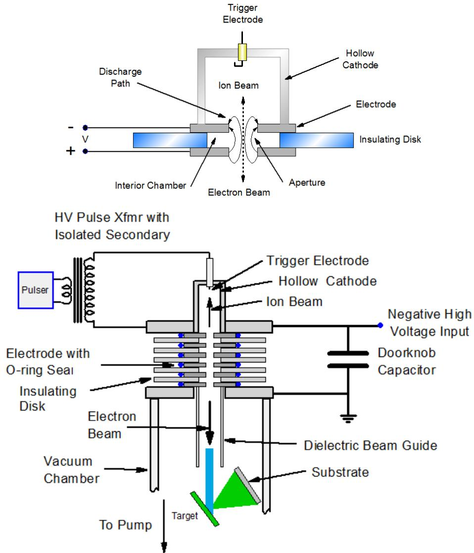
The balance of this article will be concerned with the details of the electrode assembly for my pseudospark electron source. I have generally operated this at voltages in the 30-60 kV range, free running with no external trigger.
