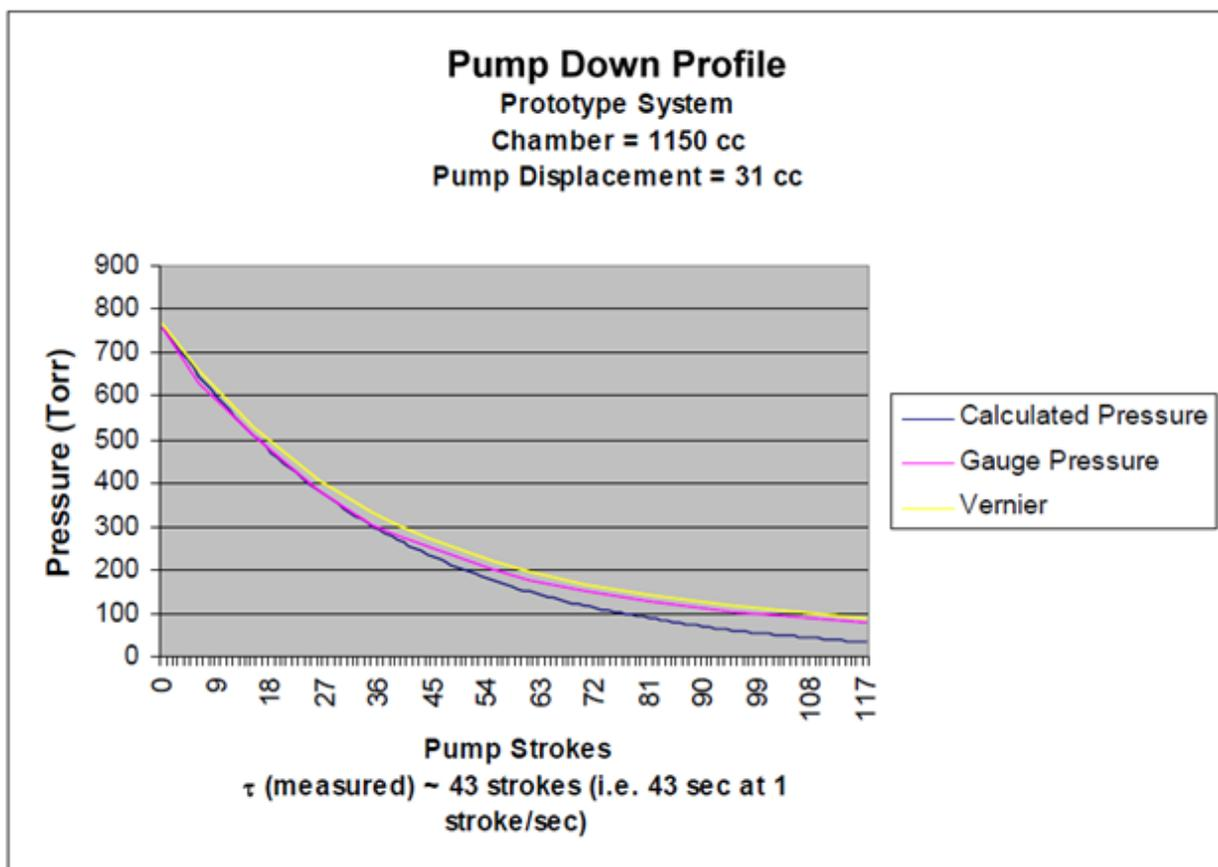
Base pressure is determined along with the upleak rate in terms of Torr/sec and standard cc/minute (sccm). The last requires a system volume determination and the application of Avogadro's Law. If there are multiple systems in a classroom, base pressures and leak rates can be compared.
