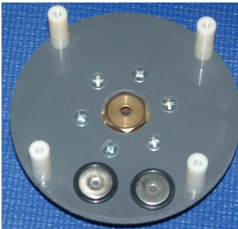
The photograph also shows two of the electrodes. The one on the left faced the cathode aperture. It has seen several thousand shots and erosion can be seen around the aperture. This is not the case with the electrodes further down in the stack.
