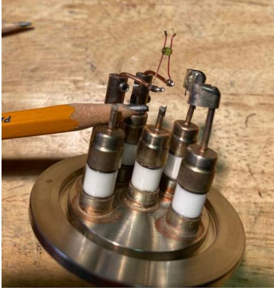
Turning to the electron source, Chuck had a KF40 base from a nude ion gauge. The photo to the left shows the base with a filament assembly that was extracted from a 3.6 volt screw base bulb. “I managed to extract [the filament] assemblies by crushing the base and glass envelope in a vise. The end result is a filament with a support bead.”
