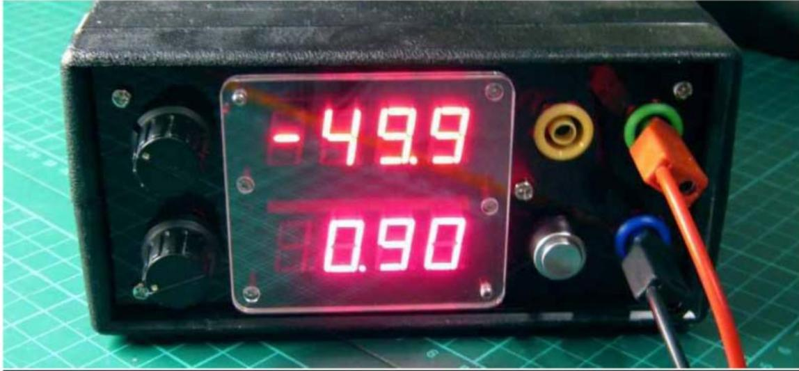
**Final unit. Grid -49.9V, Filament 0.90A**
