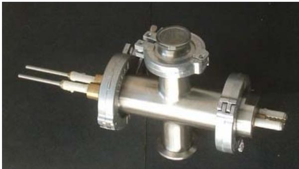
Above: Complete saddle field source showing viewport and anode rod feedthroughs.
