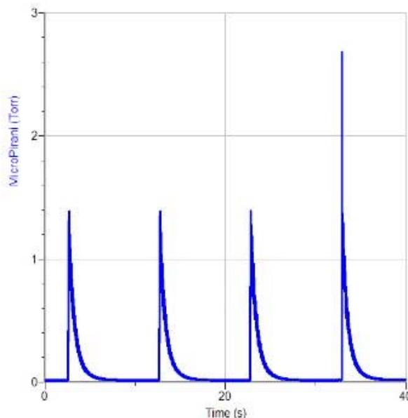
**Pulse valve testing.** The photograph at the left shows the manifold with butterfly isolation valve, vacuum gauge and fuel injector. The pulse module is at the top. The DC power supply is to the right. The plot to the right shows 4 cycles. The first three are with the isolation valve open. The 4<sup>th</sup> is with the valve mostly closed.
