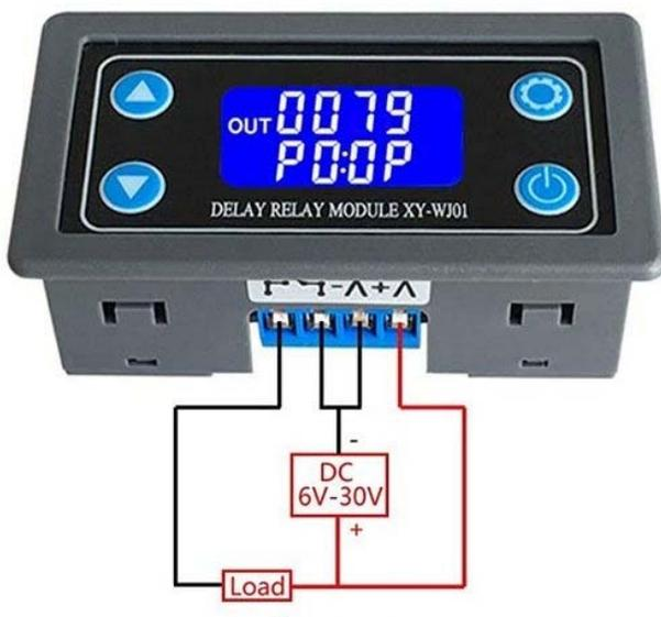
The timer can be set to on/off intervals as short as 0.01 seconds and as long as 9999 minutes. It can run in single shot or continuous modes. I'm skeptical about the low end since the switching is by relay. The relay is a Single SRD-05VDC-SL-C and the specification sheet shows an operation time of <10 msec and a release time <5 msec. I ended up setting the timer for a 10 second off period and 0.1 seconds on. This is quite conservative for the valve and relay.
