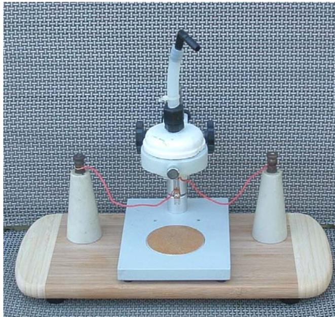
I soldered hookup wire leads to the copper foil electrodes. These are connected to 3" tall ceramic insulators. The capillary tubing is held in a Parker P4MC4 polypropylene compression fitting (1/4 tube to 1/4 M-NPT). This, in turn, is threaded into a modified PVC plumbing endcap for 1-1/2 inch threaded pipe. The body of the cap had to be turned down to 2 inches to fit the ring that was originally occupied by the microscope. The base, of course, is one of my signature bamboo cutting boards.
