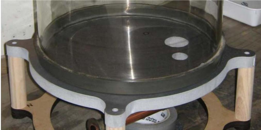
As can be seen above, the two KF apertures are a little closer that might be preferable, but by initially engaging brain rather than metal drill, it should be possible to mount both fittings without mutual interference.
