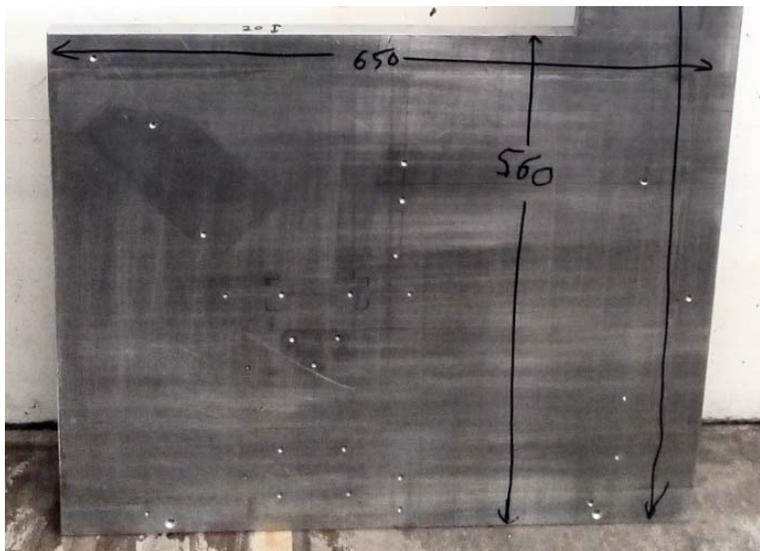
After a little contemplation, it was decided that after cutting, the plate should be mounted in each corner using M8 bolts, and should have a KF25 fitting for pumping, as well as a KF40 for electrical/gas feedthroughs. Once the required base shape had been designed, the next job was to plot it full size, and to move it around the host plate until a minimal number of holes were going to be present in the active vacuum area.
