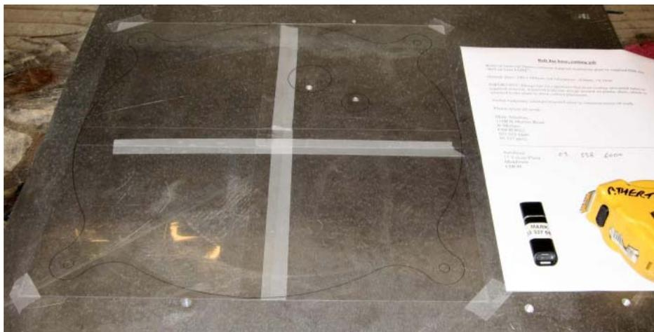
One of the other (arbitrary) design criteria was that apertures should be on a similar radius, and as far from the centre of the plate as possible - this would allow experiments to be set up in the centre of the plate.
