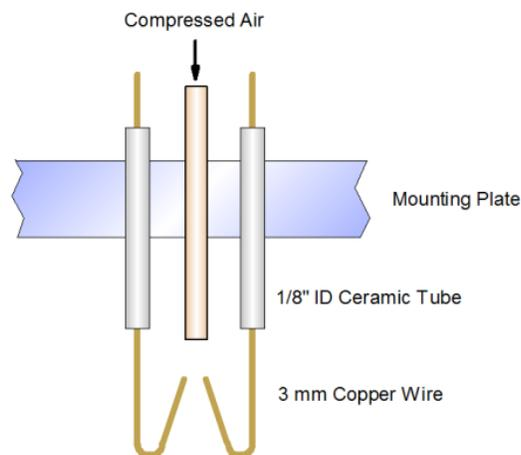
This GAD device would be suitable for producing PAW as well as for conducting other experiments such as disinfection studies.
