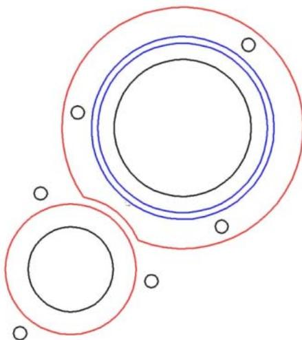
The illustration to the left shows a bottom view of standard KF25 and custom KF40 flanges. The black circles are apertures and tapped holes, red is the flange outline, blue is an O ring. The outer blue ring is also the periphery of a standard KF-40 blanking flange
