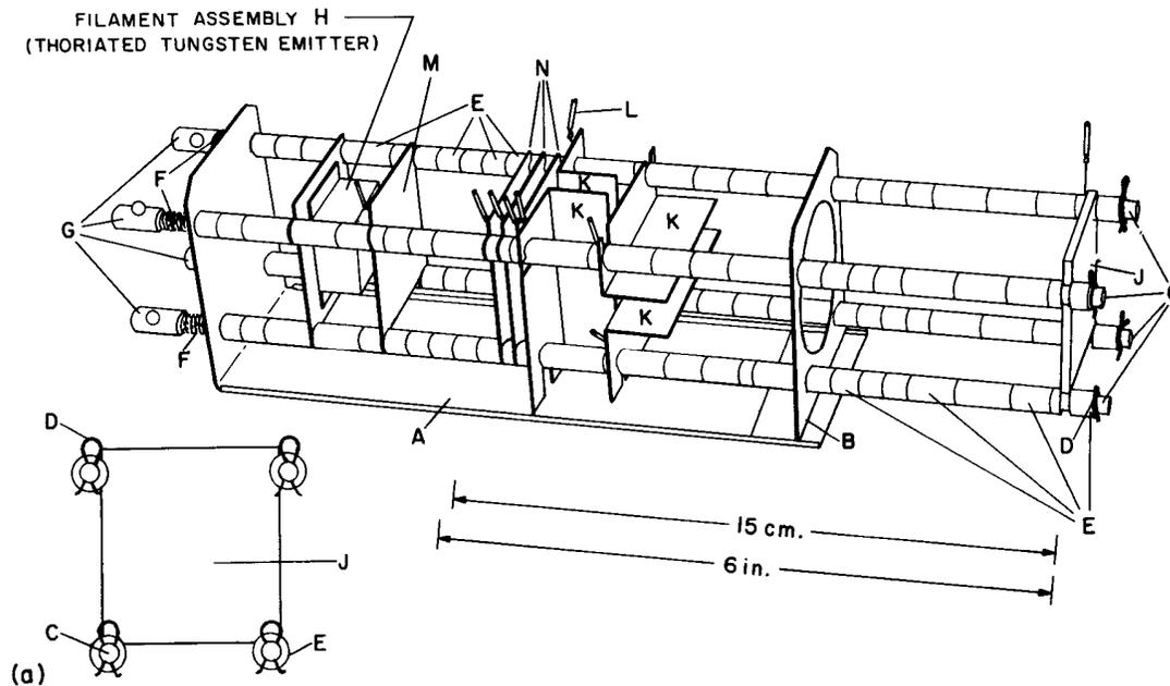
**Electron Optics Kit.** The primary features include the main frame A, ceramic rods C, retaining clips D, ceramic spacers E, compression springs F & clamps G. Electrons are generated at H, focused by elements M, N, and are deflected by plates K. The beam is detected by phosphor plate J. (a) shows the self-aligning feature. Reprinted from *Experimental Vacuum Science and Technology*, p.196, by courtesy of Marcel Dekker, Inc.
