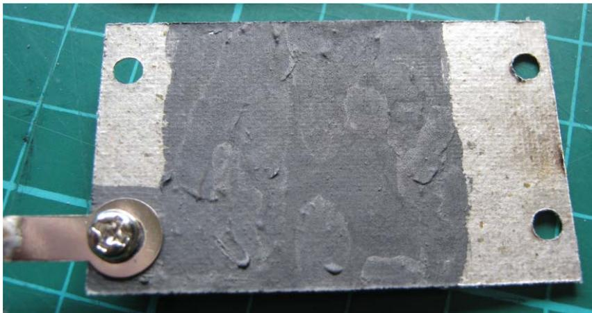
The grid was a sandwich of a fine metal mesh (possibly stainless) between a pair of mica frames, secured in two places with M3 screws. Great care was taken to remove all loose strands after the mesh was cut. The M3 bolt pushed through the hole caught on a few strands, making electrical contact. This was attached to an M3 solder tag.
