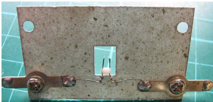
At the start of the build, it was unclear how the elements would be stacked. After some experimentation, two M3x20 screws were used (with nuts as spacers) to separate the elements. Terminal points on the filament and grid had to be moved to accommodate this new arrangement.
