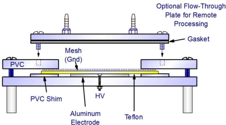
The wire mesh is not leak tight by any means. If it is desired to minimize gas leakage from the open area out the side, a bead of silicone sealant may be applied to the perimeter of the mesh before assembly. Less messy and perhaps more forgiving to disassembly would be some combination of strips of adhesive backed copper film and a gasket made from a soft elastomer such as closed cell neoprene.
