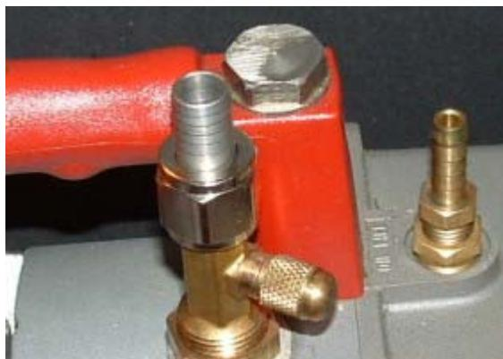
Robinair pump with 1/2” hose adapter. The 1/4” port has a cap and is used as the vent. The exhaust port to the right has been replaced with a hose connector to permit venting to the outside.
