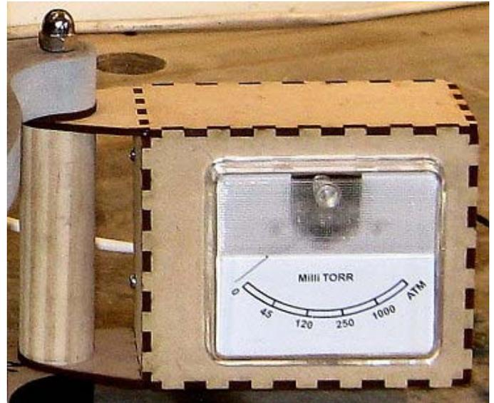
Finally, moving back to the question of making the unit battery powered. The single largest burden for the power supply is heater current, which in the case of the Varian 531 is 163mA. In its raw state, this is no mean feat for all but the most hefty battery packs. I did find some very small switching regulators based on the MP2307 switched mode power supply. These units can operate down to 4.7V on their inputs, and 0.95V on their outputs.
