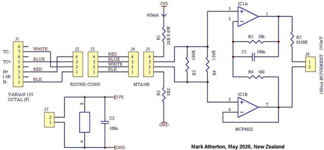
Stage gain is provided in the usual manner by R5/R6, and set to roughly 70. Early experiments indicated that the maximum output from the thermocouple was 10 mV (not 14 as expected), so R6 was replaced by a resistor / trimmer combination. Presumably the TC low output indicates that the unit needs to be degassed, or baked. This may be undertaken when hunnious-bunnious (possibly from the Latin) is out of range of the kitchen.
