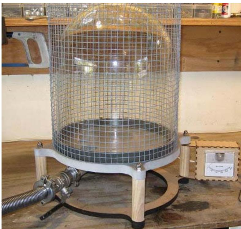
The white cable, to the rear and left of the indicator connects to the thermocouple via an octal valve (tube) socket. The black wire heading off to the right is terminated in a full size USB 'B' type plug, then onto a USB power brick plugged into mains power.
