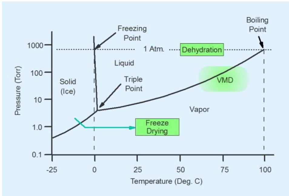
VMD has been applied in laboratory applications as well as in full production. An example of the latter would be the VMD drying of lumber. On a smaller scale, and related to Earl Rich’s effort, would be the 2015 paper by Monteiro *et al.* [1]. They described a VMD system based on a domestic microwave oven. The motivation was to have a lab-scale apparatus that would be simple and economical. The figure below is a simplified diagram of the apparatus, based on the authors’ description.
