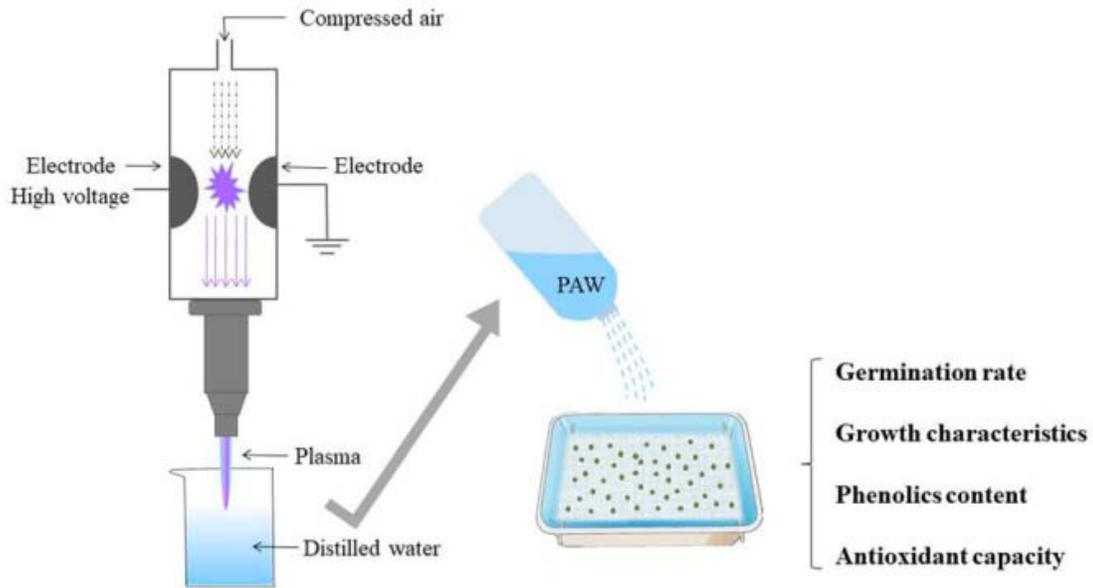
**PAW Experimental Set Up.** From Fan *et al.* [2], *Effects of plasma-activated water treatment on seed germination and growth of mung bean sprouts*. Open source document.
