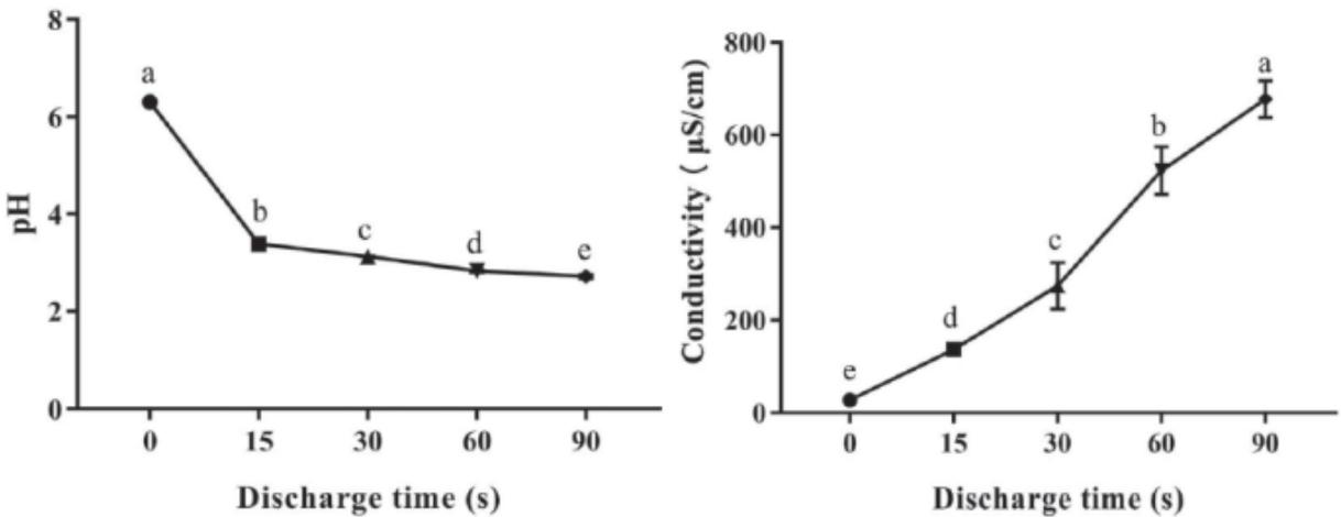
**Plots for pH and electrical conductivity.** From Fan *et al.* [2]. Open source document.
