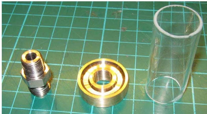
**Swagelok fitting, brass end, and plasma tube**
