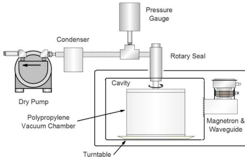
The attributes are much the same as that of Earl Rich’s wood drying apparatus. The most significant change is the use of the oven’s turntable to rotate the vacuum vessel containing the product. This required the addition of a rotating vacuum seal. The authors also optimized the waveguide.
