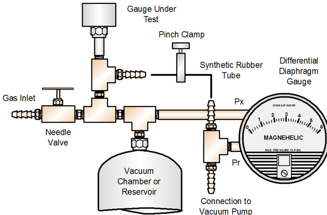
The manifold was constructed using ¼" brass threaded pipe fittings between the pump fittings and the chamber. Other fittings, such as the gauge ports and the needle valve, had 1/8" fittings so adapters had to be used at these points. The valve that served to isolate the reservoir and measurement side from the reference side and pump was a short length of ¼" id synthetic rubber tubing with a pinch clamp.
