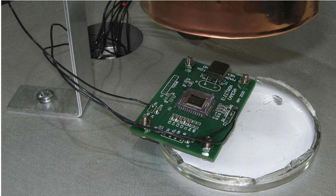
Imager assembly, next to the dismembered CRT faceplate
