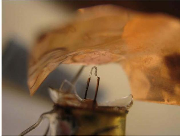
Tungsten filament and copper anode
