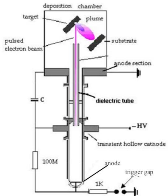
The voltage across the dielectric section accelerates the electrons escaped from the cathode and the so-called channel discharge occurs.
