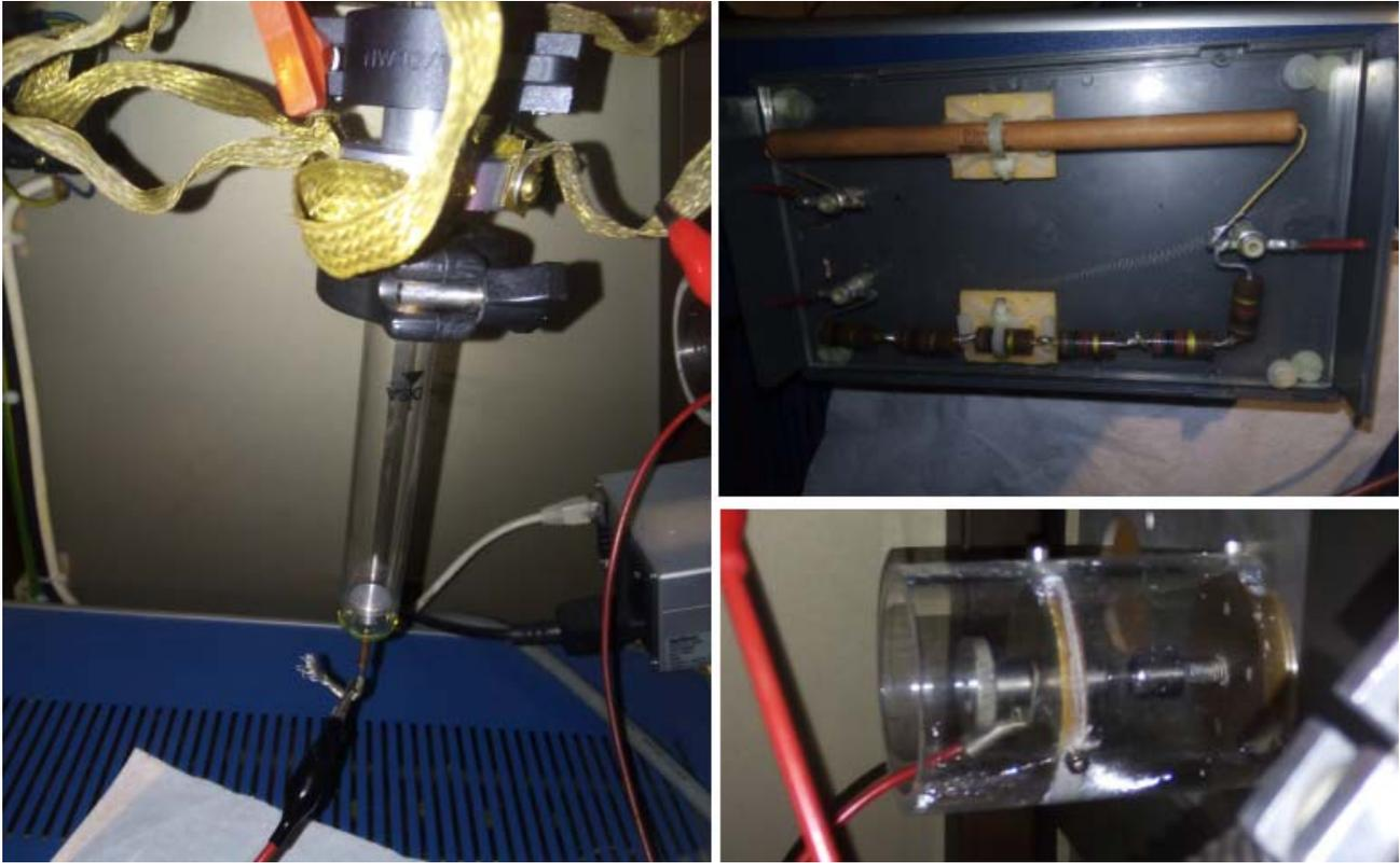
Above left - Vacuum bulb with anode, hollow cathode and connections to the capacitors; top right - The resistor box with cover removed; bottom right – the adjustable spark gap. Photographs courtesy of Dr. Patrizio Graziosi.
