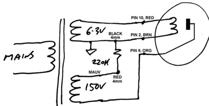
Thermionic Diode test fixture
