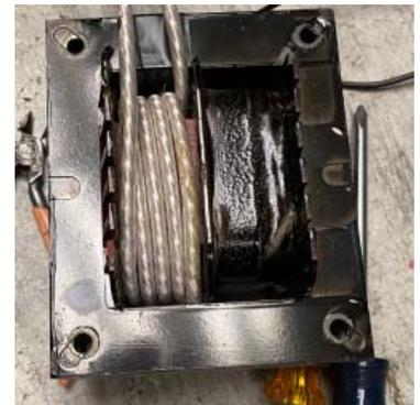
I think a 5 volt, 20 amp tube transformer would work well. A Variac is needed to control the filament temperature.
