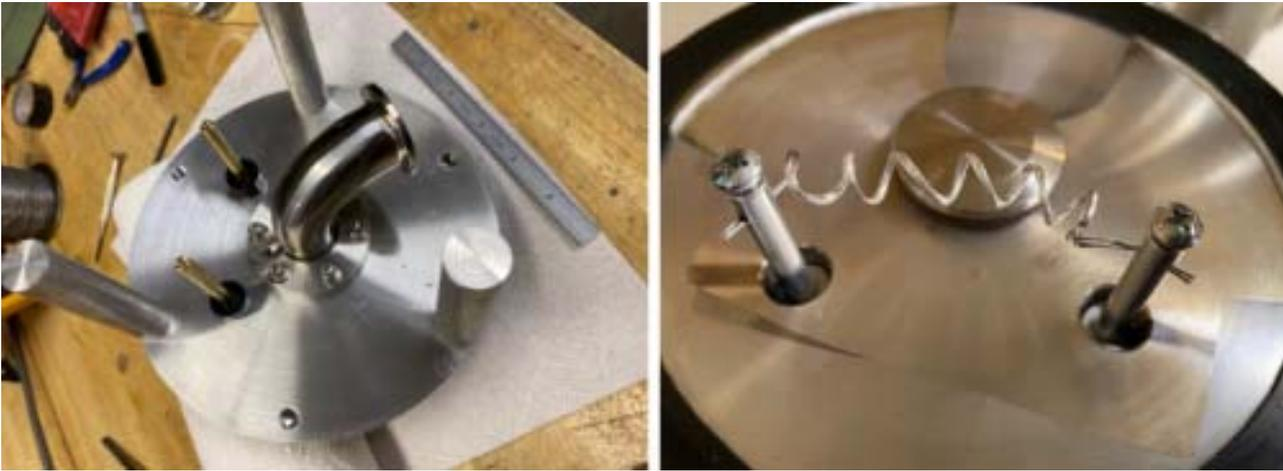
A gasket for the bell jar was cut from sheet rubber, believed to be EPDM. Silicon grease was used on both sides of the gasket because EPDM does not tolerate petroleum based products. A #5 stopper was used in the top hole with a ¼-inch brass rod and aluminum disk to attempt some plasma cleaning. A 10 kV oil burner ignition transformer was used as a power source for plasma cleaning.
