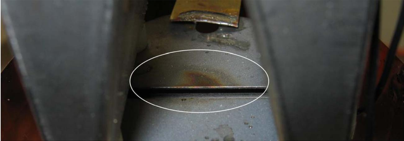
Electron heating of G24 electrode within the electron gun
