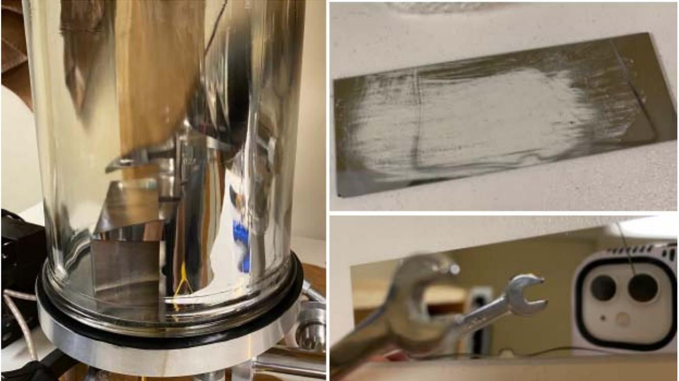
The photograph above left shows the coating on the inside of the bell jar. To the right are two photographs of microscope slides that have been coated. The top right photograph was done at  $10^{-4}$  Torr with no plasma cleaning. It did not adhere well and the coating rubbed off with a paper towel. The one below was coated at  $10^{-5}$  Torr with plasma cleaning. It made a perfect mirror coating.
