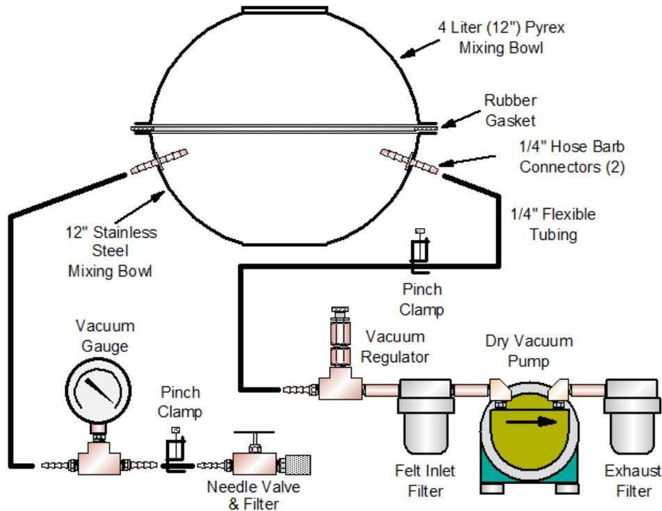
Holes can be cut in the stainless bowl to permit the incorporation of feedthroughs. I used 1/4" brass hose barbs, epoxied in place. I was a bit concerned about the ability of the steel bowl to withstand vacuum but the only effect was a very slight bowing of the flat bottom. There are probably a lot of other applications where a simple chamber setup like this would be handy.
