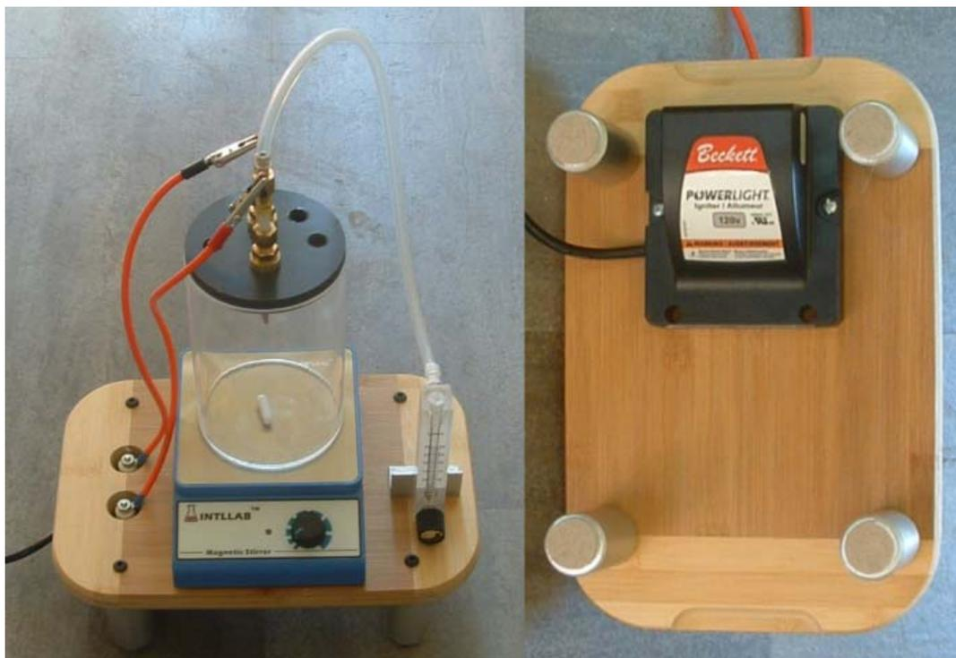
Above are two photographs of the assembly. I built it on one of my signature bamboo breadboards. The acrylic chamber sets on a magnetic stirrer. There are four standoffs that serve as feet. These provide clearance for the electronic oil burner transformer that is mounted on the underside. Connections to the GAD electrodes are provided by high voltage silicone insulated
