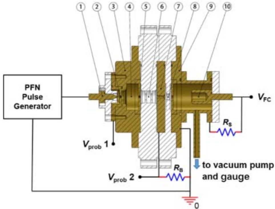
Post acceleration structure of the pseudospark sourced electron beam source
