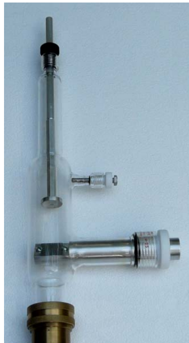
Figure 4 - Tube Configured for X-Ray Production
